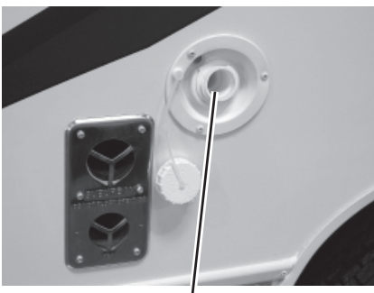
Fresh water tank fill
